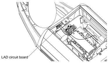
Figure 5-5. The laser aiming device circuit board.
