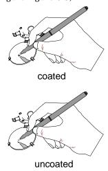
Figure 6-5. You can easily tell which side of a dichroic is coated by placing a pen or other object near the surface; on the coated side, the reflection from the object will appear to touch the object.
