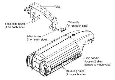
Figure 1-1. Identifying yoke components.
