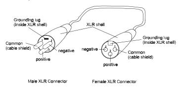
Figure 2-3. Properly-constructed data cabling.
