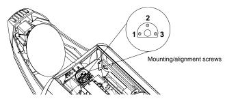
Figure 6-27. The laser aiming device assembly has three screws that can be used to adjust the position of the laser.
