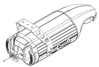
Figure 6-14. Removing the lamp assembly from the fixture.
