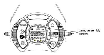
Figure 6-13. Loosening the lamp assembly screws gives you access to the fixture lamp.
