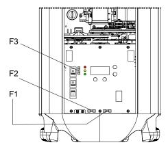
Figure 6-2. Locations of the three fuses on the circuit board.
