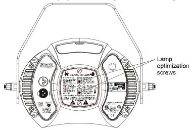
Figure 6-18. Lamp optimization screws.
