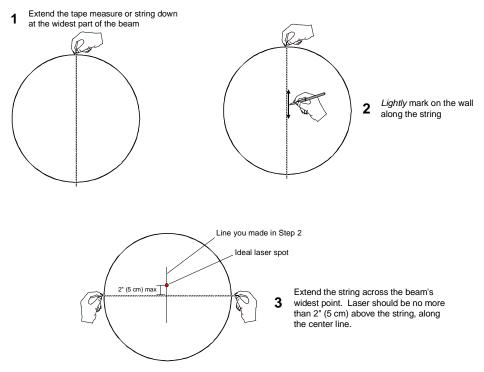
Figure 6-26. Locating the center point of the projected light beam. The laser should be no more than 2" (5 cm) above the center.
