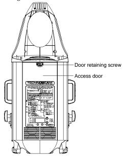
Figure 6-19. Opening the fixture's access door.
