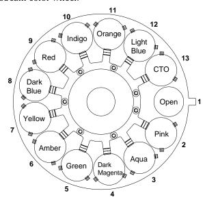
Figure B-2. Factory configuration of the Technobeam color wheel. Technobeam rotating effects wheel:
