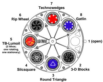
Figure B-1. Factory configuration of the Technobeam rotating litho wheel.
