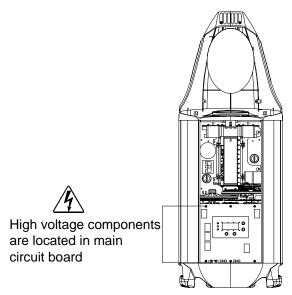
Figure 6-24. High-voltage component location.
