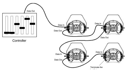
Figure 2-6. Connecting fixtures to a controller. Make sure you terminate the last fixture in the link.
