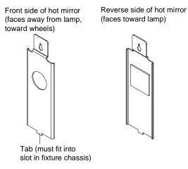
Figure 6-22. Clean both sides of the hot mirror glass.
