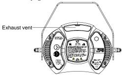
Figure 2-13. Location of the fixture's exhaust vent.
