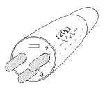
Figure 2-4. Constructing a data cable terminator.
