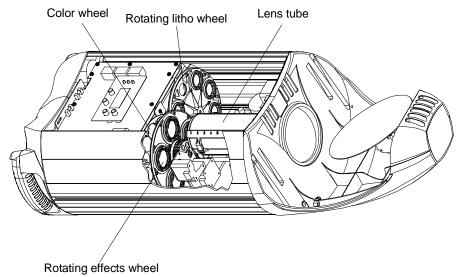
Figure 6-3. Location of the wheels in Technobeam.
