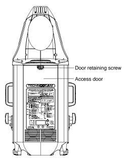
Figure 5-3. Removing the access door.
