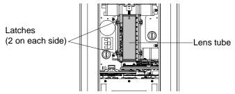
Figure 1-6. The lens tube contains the zoom lenses.
