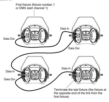
Figure 4-3. When you set up fixtures for synchronized playback on a DMX 512 link, one and only one fixture **must be** fixture number 1 or DMX start channel 1. The last fixture on the link must be terminated.
