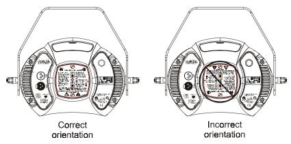
Figure 6-17. You can look at the lamp label text to make sure the lamp plate is oriented correctly; incorrect orientation can result in damage to the fixture and the lamp.
