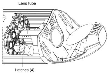
Figure 6-21. The lens tube contains the zoom lenses.
