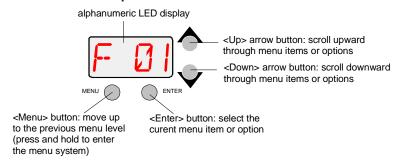
Figure 3-1. Technobeam navigation buttons.
