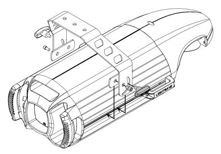
Figure 1-2. Installing the yoke on the fixture.
