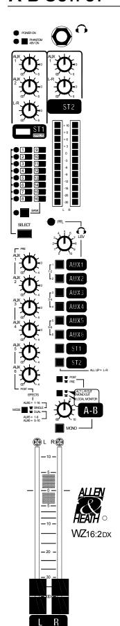
The A-B output is an additional stereo/mono output that can be uniquely configured as either a **separately controllable mix** output, or a **local loudspeaker monitor** feed.
