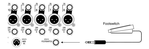
A footswitch can be plugged into the rear panel FOOTSWITCH socket to control the effects. A passive momentary action switch type as commonly found in music stores is required. However, it may be necessary to modify the cable by fitting a 3-pole 1/4" TRS (tip, ring, sleeve) jack plug and wire it according to the required function as follows:
