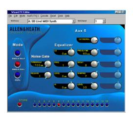
Individual effects parameters can be changed and these loaded back into the mixer to overwrite the factory default settings. This is best done using the Allen & Heath **MixWizard FX Editor** software running on a PC with MIDI port. You can download this free from the Allen & Heath web site.
