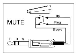
A momentary action dual-pole footswitch that shorts sleeve to tip of jack through one pole and (separately through the other pole) sleeve to ring of jack acts as an 'effects mute' toggle switch. If a single pole switch is used, it will not work correctly.
