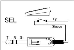
A momentary action footswitch that shorts sleeve to tip of jack will duplicate the front panel 'Sel' switch to select the effects type.
