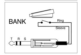
A momentary action footswitch that shorts sleeve to ring of jack will duplicate the front panel 'Bank' switch to toggle between the two banks of effects.
