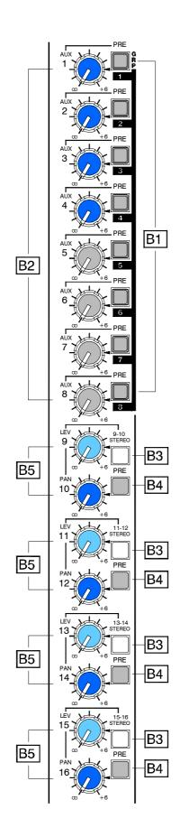
These controls send the channel signal to the audio groups 1-8 and aux sends 1-16. They are the same for both the mono and stereo channels.
