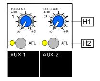
These are the masters for the channel post-fade aux sends 1-8. They are normally used as sends to effects processors such as reverb. Note that the channel send rotaries B2 are dual element controls that simultaneously send the post-fade signal to these rotary masters and the pre or post-fade signal to the fader masters F.
