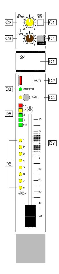
C1 MAIN MIX. A single switch routes the channel signal to the 3 output main mix. Its balance and image within the L, R and C outputs is determined by the BLEND and PAN controls.
