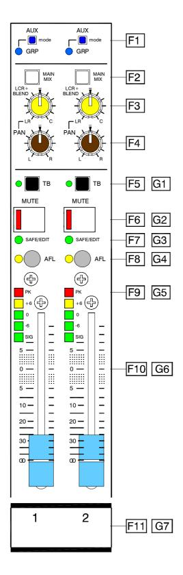
F1 AUX/GRP MODE. This switch configures each fader master 1 to 8 as either an audio group or an auxiliary send. It is underpanel to protect it from accidental operation. Use a pen or pointed implement to select the required setting. The default up position is flush with the panel.
