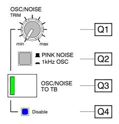
WARNING: The generator is capable of producing a high level continuous signal. To avoid damage to the speakers check that the generator and output levels are turned down before you route the test signal to the outputs.
