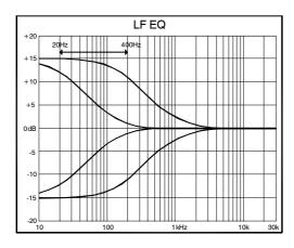
A7 **EQUALISER**. The channel equaliser provides adjustment of 4 independent frequency bands. Each has cut/boost and frequency sweep controls. HF and LF are shelving. HM and LM are fully parametric peak/dip with Q control.
