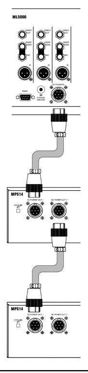
The **ML5000** console range is supplied with the **MPS14** power supply unit. A second **MPS14** may be connected through the first as a redundant (backup) supply.
